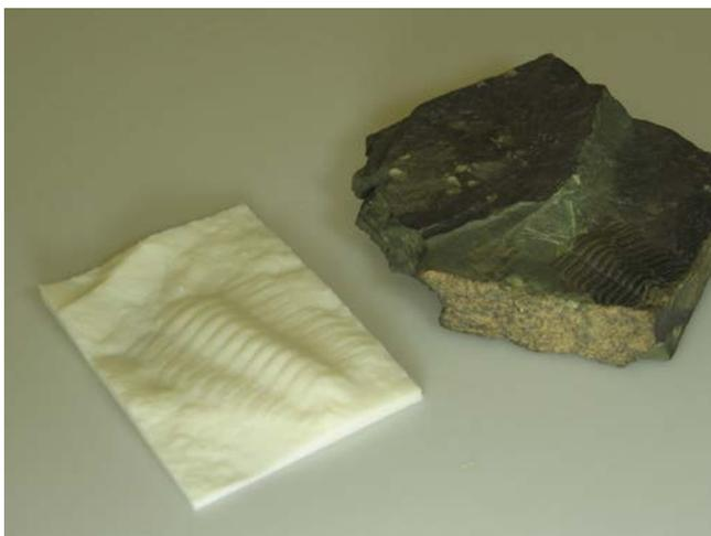
Figure 5. Original fossil and its enlarged replica created using 3D printer
