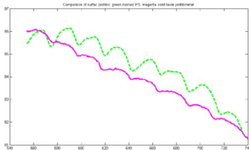
Figure 4. Comparison of the results from laser profilometry (magenta line) and photometric stereo (green dashed line) for selected line on the object (red line in the upper part of the figure).
