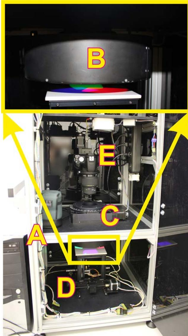
Figure 2. Device for 3D digitisation. The illumination part is shown in the inset. A – modular frame, B – RGB illumination, C – rotating stage, D – positioning table, E – DSLR camera.
