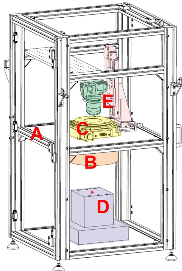
Figure 1. Schematic drawing of device for 3D digitisation. The illumination part is shown in the inset. A – modular frame, B – illumination, C – rotating stage, D – positioning table, E – DSLR camera.
