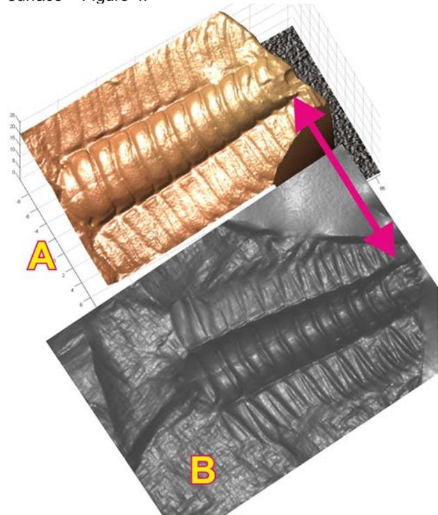
Figure 3. Comparison of the 3D model of trilobite as rendered through (A) laser profilometry and stereo (B) photometric. Arrow points to difference in details.
