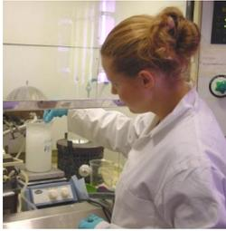
Figure 7. Surface treatment by alkaline etching in the lab: suspending the test cubes in the sodium hydroxide solution.
