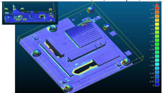
Figure 18 Comparison Arius3D scan vs Nikon MMD. Scale covers a +/- 0.5mm range and demonstrates systematic discrepancies between the two sets of measurement data. (Cloudcompare, <http://www.danielgm.net/cc/>)
