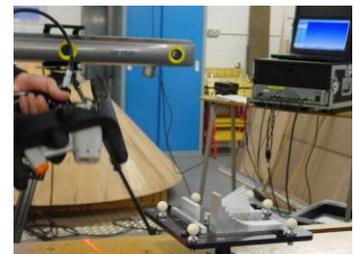
Figure 12. Nikon handheld MMD and Krypton K610 Camera for 3D scanning of test object. Specification are given in (Hess & Robson 2010) ([www.nikonmetrology.com](http://www.nikonmetrology.com))
