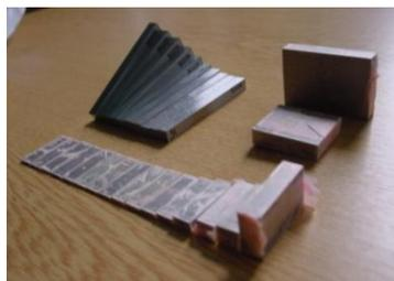
Figure 1. Mock-up of test object: set of Steel Slip Gauge Set M32, Calibration Grade 1 and Angle Block Set, length gauges to test step height and as length bar ([www.msclindustrial.co.uk](http://www.msclindustrial.co.uk)).
